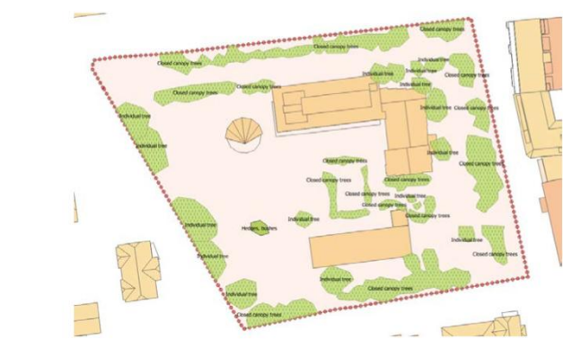
Figure 4. BGF-QGIS map of the demonstration locality (property of the County Governor, Ås, Norway; tutorial locality of the BGF-QGIS documentation) after digitising blue-green surfaces and additional qualities, with final BGF = 0.871 (top), and the corresponding tree-canopy and vegetation layer (bottom). Reproduced from Horvath et al. [7], NINA Report 1445, which may be freely cited with acknowledgement of the source.
